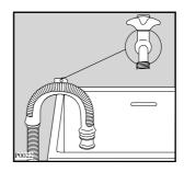
D) Place the discharging hose in a washbasin or sink with the aid of the bent piece delivered separately. The bent piece has to be entered into the tube's mouth in order to assure the support. Aforesaid piece allows the hose to be fixed to the wall by means of an opening on the upper part and that way the hose does not move and its falling is avoided.
